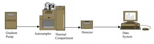
Figure 3 HPLC System Configuration
