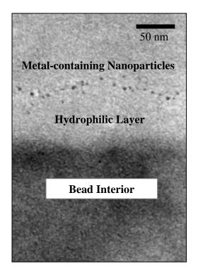
Figure 1 TEM of Cross-section of a Metal Charged IMAC Phase
