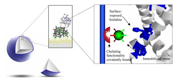
Figure 2 Theoretical Interaction of a Protein with the Dionex ProPac IMAC-10 Phase
